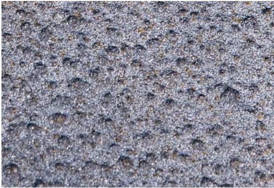
As-sprayed surface .050" (1.27mm) thick, using cored wire.
