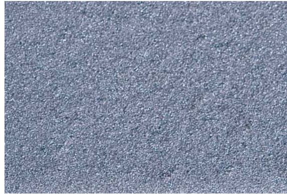
As-sprayed surface .225" (5.72mm) thick, using ArcMelt's composite wire.
